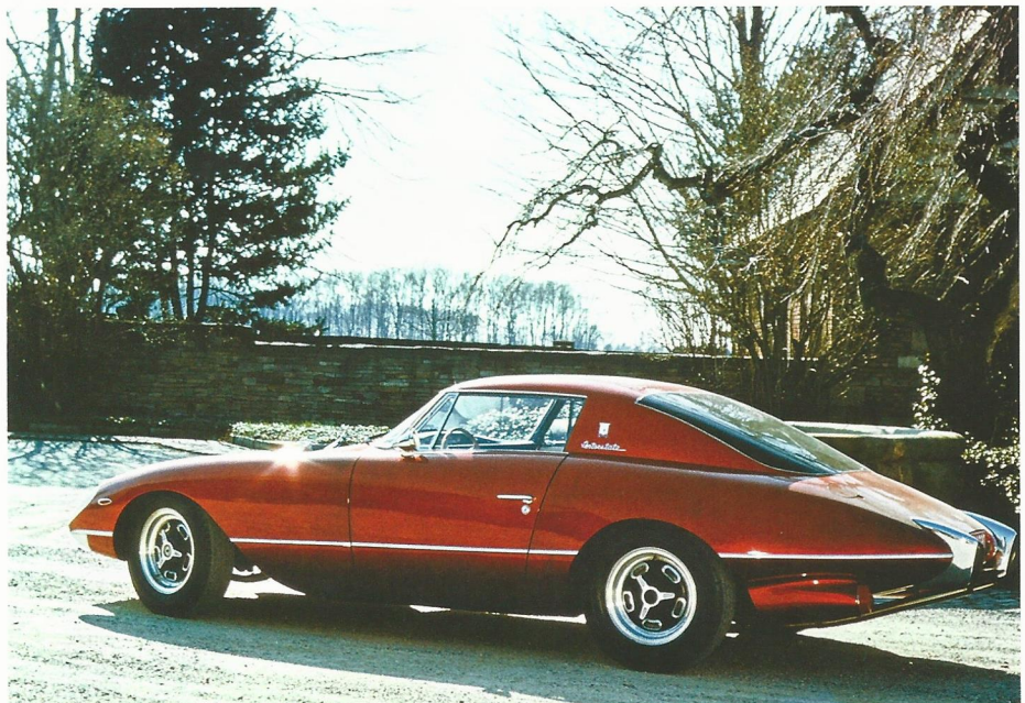
Bosley built his second car in the mid-1960s, using the chassis from a Chevrolet Corvette SR-2—one of three that were built for racing in 1956. Designed for the fast new roads that were springing up across the United States, the Bosley Mark II Interstate was fitted with a 345-bhp Pontiac V8 and a 4-speed manual transmission.
