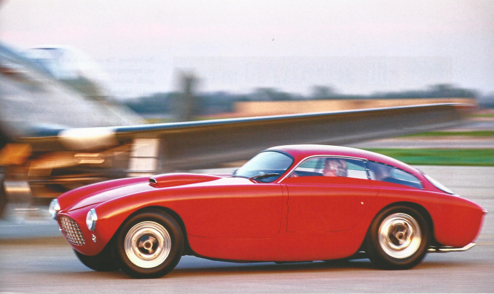
The 1953 Bosley Mark I prototype was built by Richard Bosley, a horticulturist from Mentor, Ohio. The car featured a steel tube frame; Ford, Mercury and Lincoln mechanicals; and a Chrysler Hemi engine, all clothed in a handlaid fiberglass body.
