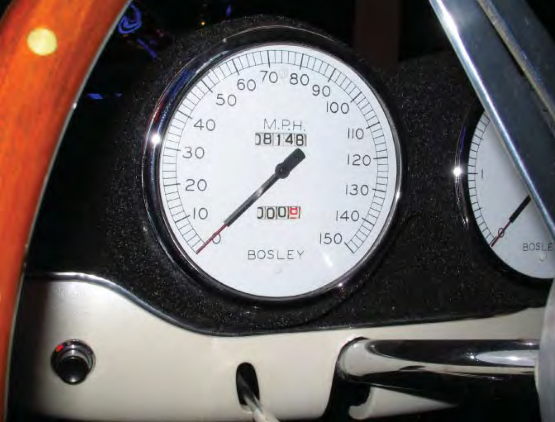
Speedometer and tachometer were special-built from Ford police instruments.
